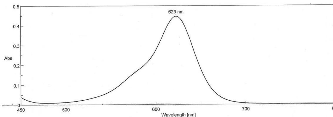
Figure no. 1  $\lambda_{\max}$  graph for Metoclopramide hydrochloride with chloramine-T and malachite green
